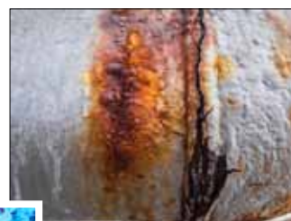
Right: SCC in a pipe weld
