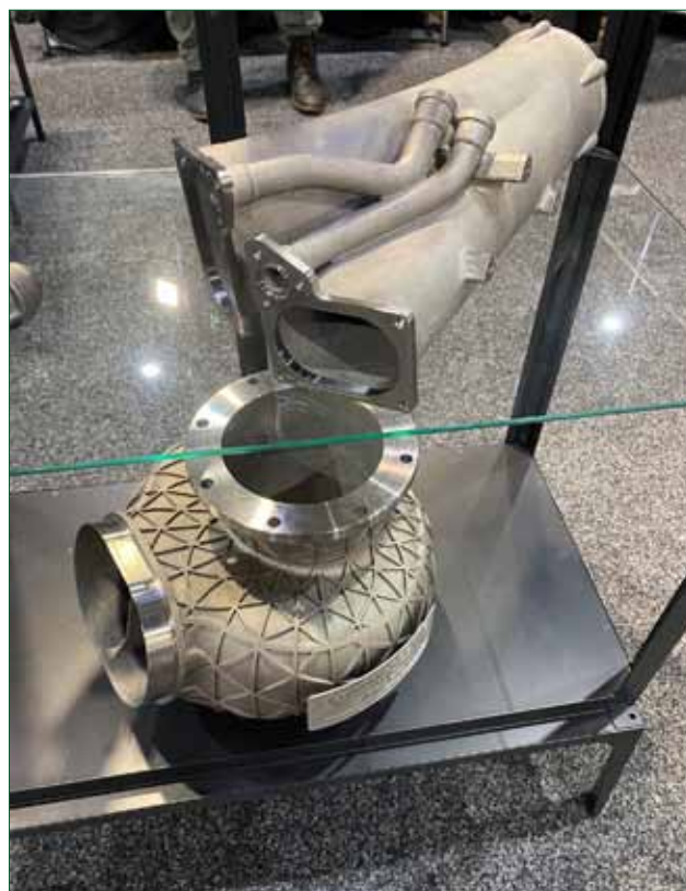
Complex titanium metal parts manufactured by additive manufacturing (3D-printing).
