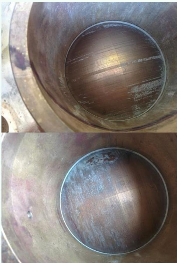
Figure 4: Hull valves – calcareous deposit from on valves which were seizing closed.
