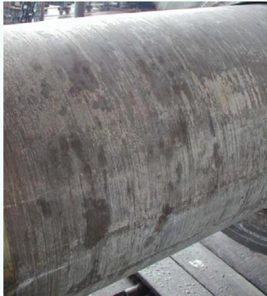
Figure 3: Propeller shaft bearing with a calcareous deposit (above) and at x600 magnification (right).
