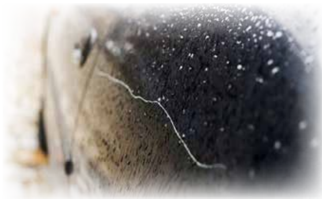
A self-healing coating uses sunlight to repair scratches on a car finish
