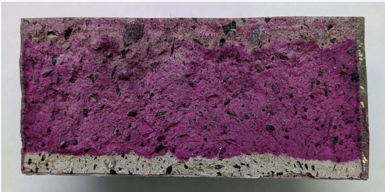
(Above) Figure 3: Cross-section of concrete sample treated with the Realkalization Solution on top section following accelerated carbonation testing for 8 weeks. Light colouration indicates carbonated concrete which maintains high alkalinity (measured as pH 11.4 by ground sample leaching method), while darker areas indicate non-carbonated concrete.
