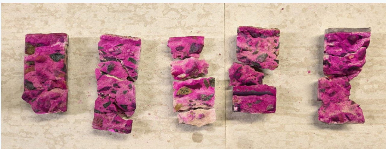
(Above) Figure 3: Cross-section of concrete sample treated with the Realkalization Solution on top section following accelerated carbonation testing for 8 weeks. Light colouration indicates carbonated concrete which maintains high alkalinity (measured as pH 11.4 by ground sample leaching method), while darker areas indicate non-carbonated concrete.
