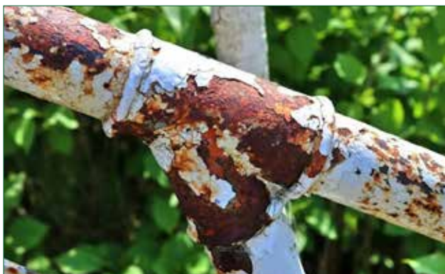
Coating failures lead to steel rusting
