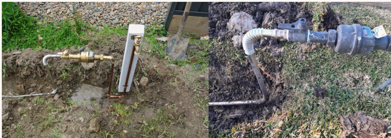
Figure 7: SPCT as installed, left, and right, exhumation after 3.5 years exposure. Note patina on copper alloy fittings (right) showing corrosive atmosphere present at site.
