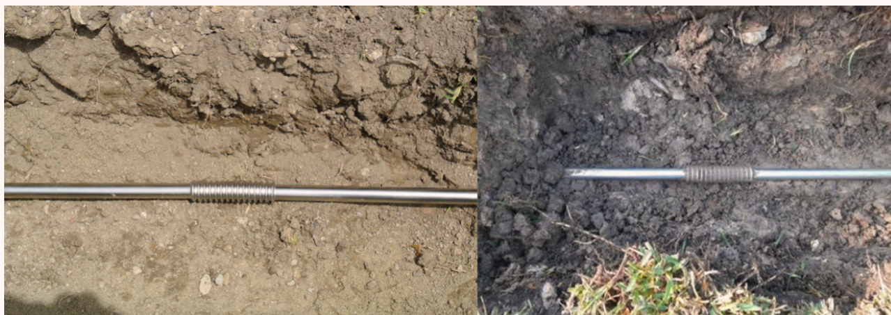
Figure 8: SPCT as installed, left, and right, exhumation after 3.5 years exposure. Note that stainless tube on right still bright and uncorroded despite burial in corrosive clay soil without granular backfill.
