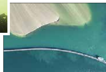
Right: Aerial image of Ōhau Channel diversion wall appears to show sediment leakage
