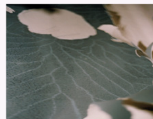
Fig20B: Base coat revealed showing virtually no adhesion to primer
