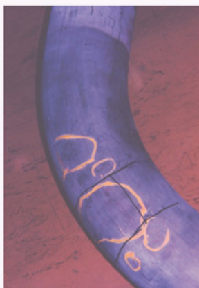
Fig 16A: Cracks ringed
