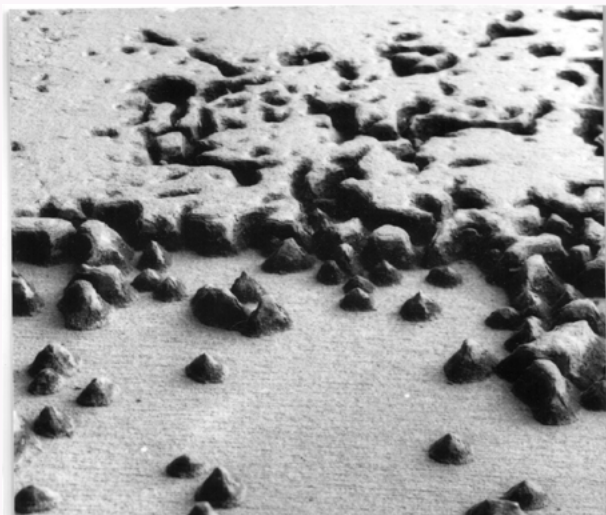
Fig 19: Aluminium sheet after 14 hours in mid strength NaOH
