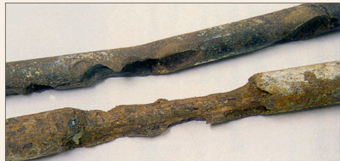
Figure 5. Example of marked localised pitting (macrocell) corrosion and section loss (corrosion penetration) of steel reinforcement. Here pits would have started out narrow but with time have coalesced to result in section loss over a greater (anodic) area.
