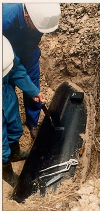
Figure 7: Site 2, Horsham, 1991, undertaking the bond adhesion test on the 724mm diameter, 14 year service pipe.
