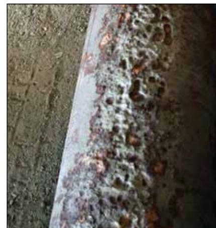
Pitting of cast iron water pipe (photo courtesy Matt Dafter).
