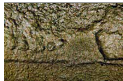
SEM view of pipeline under-deposit corrosion.
