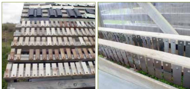
Figure 1: Rack with coupons on Muriwai Beach/New Zealand.
