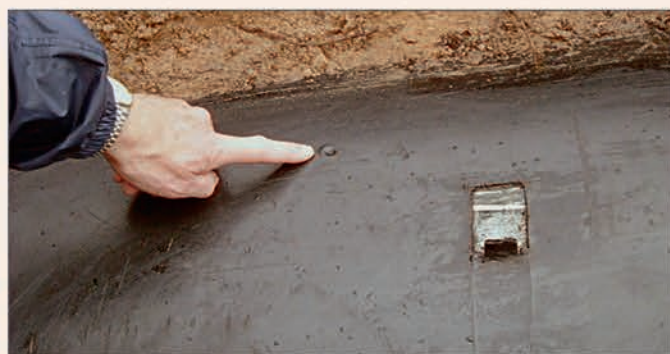
Figure 10: Site 3, Geelong, 2004. Buried pipe showing impact test indentation and bond test.
