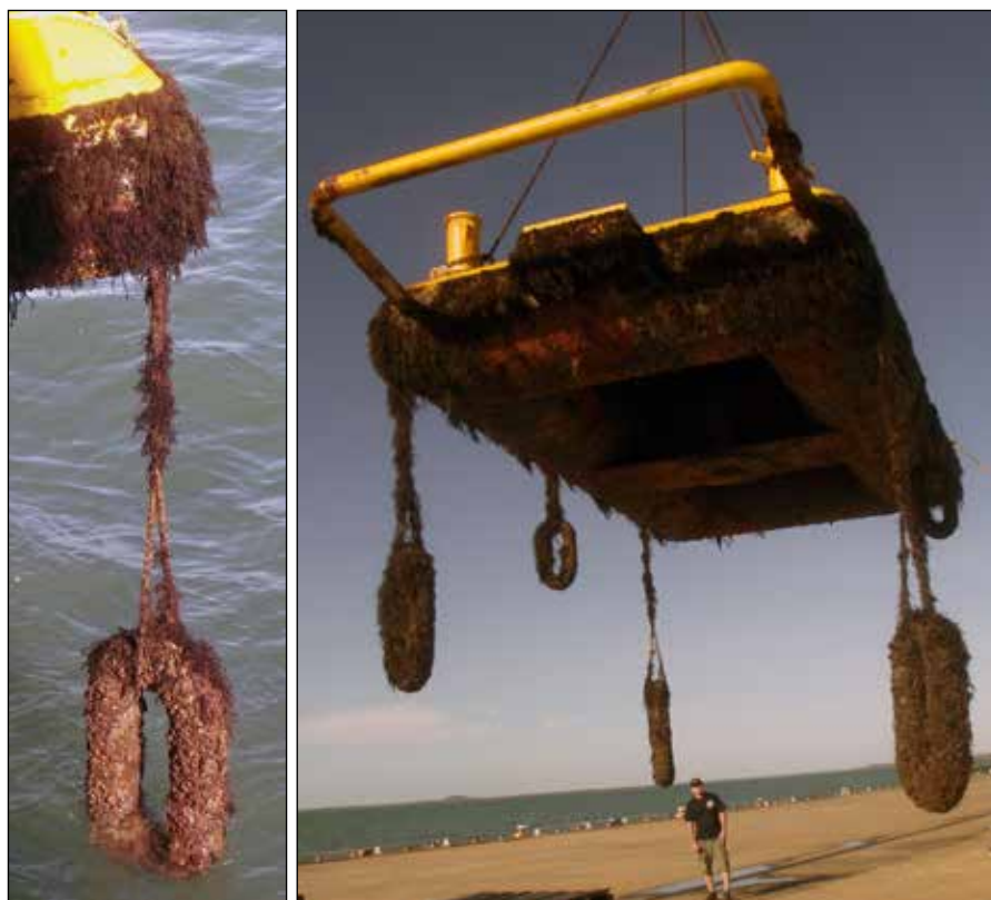
Recovery of 150 mm diam. mooring chain at Darwin after 2 years exposure.
