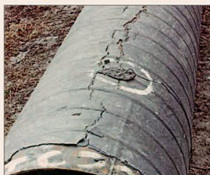
Figure 1: Coal tar enamel coating showing crown cracking on 914mm pipeline - 1971.
