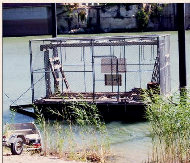
Figure 14: Murray River Pontoon for immersion exposure.
