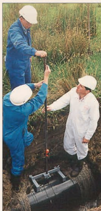
Figure 6: Site 1, Horsham, 1991, showing the 8 year service, 724mm pipe, and preparations for impact testing.
