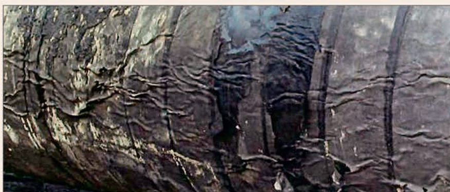
Figure 2: Coal tar enamel coating showing coating deformation on 914mm pipeline - 1971.
