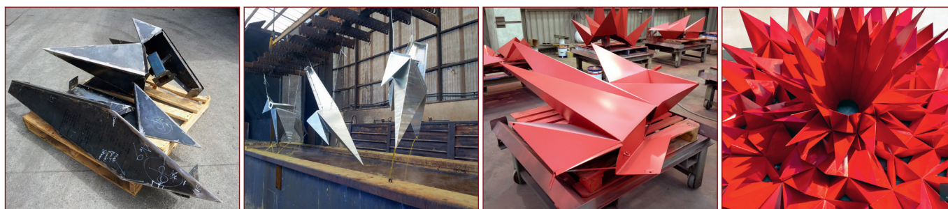
Figure 3: The Moment by Damian Vick, showing the four key stages of fabrication, galvanizing, painting and the final structure in place. This aesthetic sculpture is an example of a complex shape with sharp edges and is therefore suited to a duplex coating.
