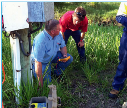
Allan Sterling showing Josh Logan how to measure earthing potentials.
