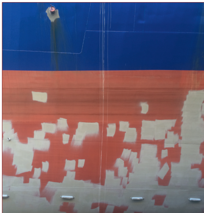
Tasport's Korimul Tug refurbishment over spot blasted surface with UHWJ.
