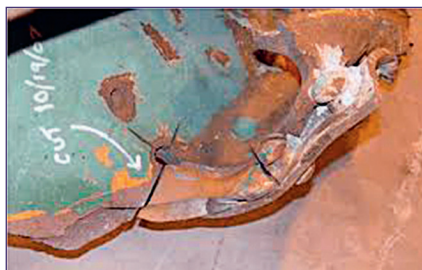
Figure 5. Bridge I35W steel gusset plate showing cracking and corrosion [7].
