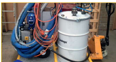
A Rhino Linings high-pressure, plural component, spray machine on a travel pallet, with drums in banded sections to contain minor spills.
