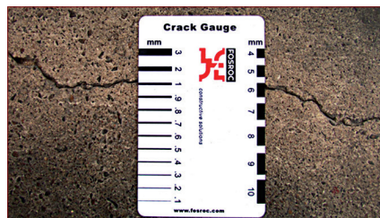
Concrete Cracks provide easy access to corrosive agents.
