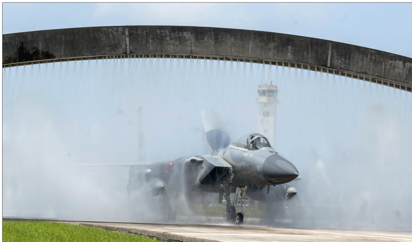
An F-15 Eagle goes through a birdbath at the Kadena Air Base in Japan. The birdbath is a vital component of maintaining the longevity of Kadena's fighter aircraft. The birdbath prevents corrosion from building up on the aircraft. Photo courtesy of Airman 1st Class Lynette M. Rolan, U.S. Air Force
