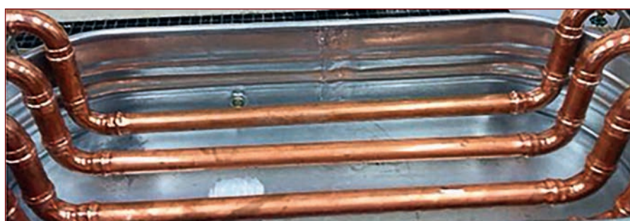
Figure 2: Test trough with bare copper pipes.
