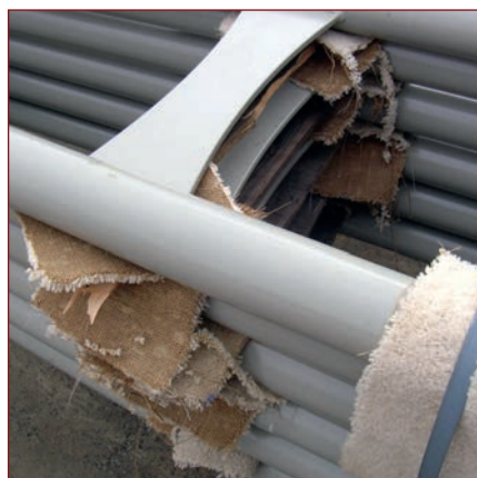
Even after curing, paint coatings must be handled and transported carefully.
