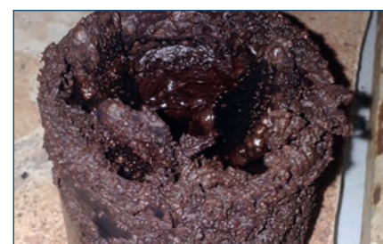
Corrosion of 316SS in molten salt.
