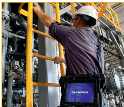
An iPlex NX videoscope can be taken to areas that have restricted access.
