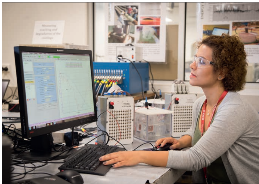
Student Fariba Mahdavi takes measurements on a defective coated probe to study cathodic disbondment of coatings.
