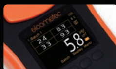
Four Bresle patch equivalent readings in 2 1/2 minutes
