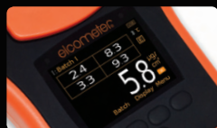
Four Bresle patch equivalent readings in 2 1/2 minutes
