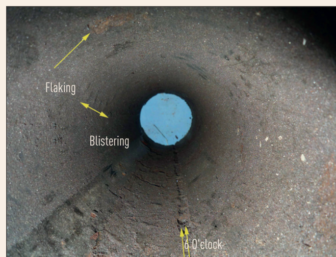
Examples from typical corrosion patterns; 6 o'clock corrosion due to water drop out, flaking and blistering due to formation of porous & instable scales.
