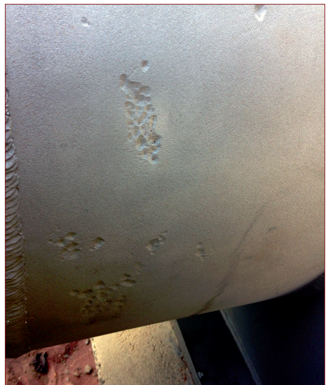
East End Corrosion.
