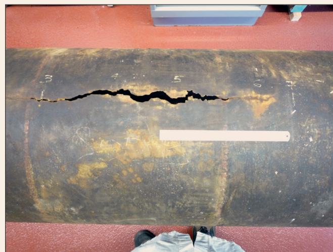
Extreme corrosion and associated wall thinning can lead to dramatic loss of primary containment (LOPC) failures in the field.
