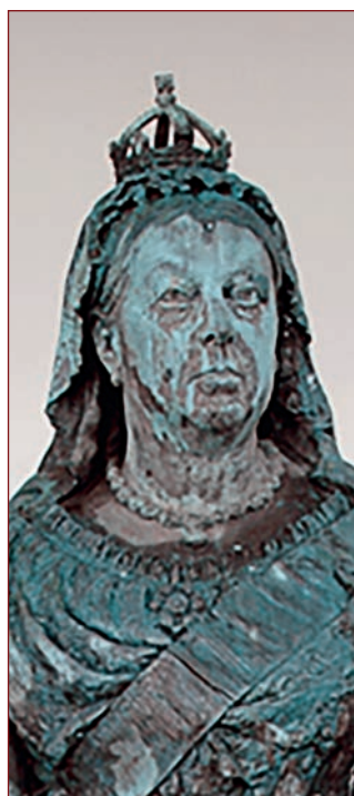
Figure 4. Queen Victoria statue showing extensive corrosion on the bronze surfaces.
