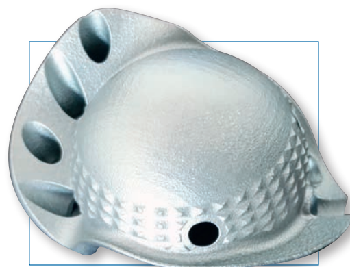
3D printed acetabular cup, produced by selective laser melting of Ti-6Al-4V. This specific cup has been implant into a patient in Australia, produced at Monash University.
