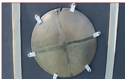
Figure 15. The bronze disc after exposure to a severe marine environment for 3 months.
