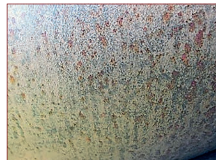
Figure 11. Rust spots and streaks that developed on the polished surfaces of the silicon bronze sculpture.
