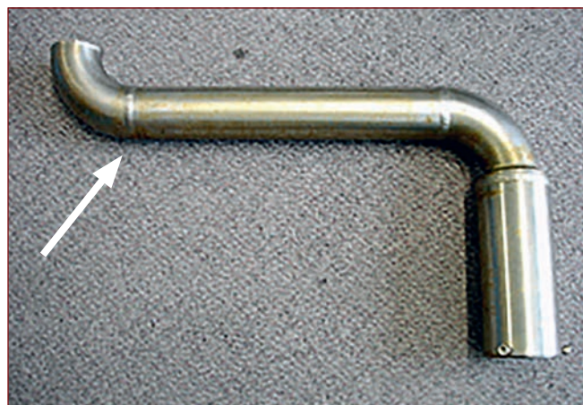
Figure 8. 316L stainless steel support pipe elbow on sculpture cone. Cracking occurred at pipe weld (arrowed).
