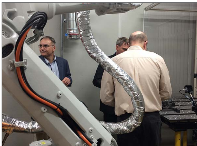
This robotic arm is programmed to apply cold spray technology to repair surfaces of corroded aircraft parts. Credit: University of Akron.
