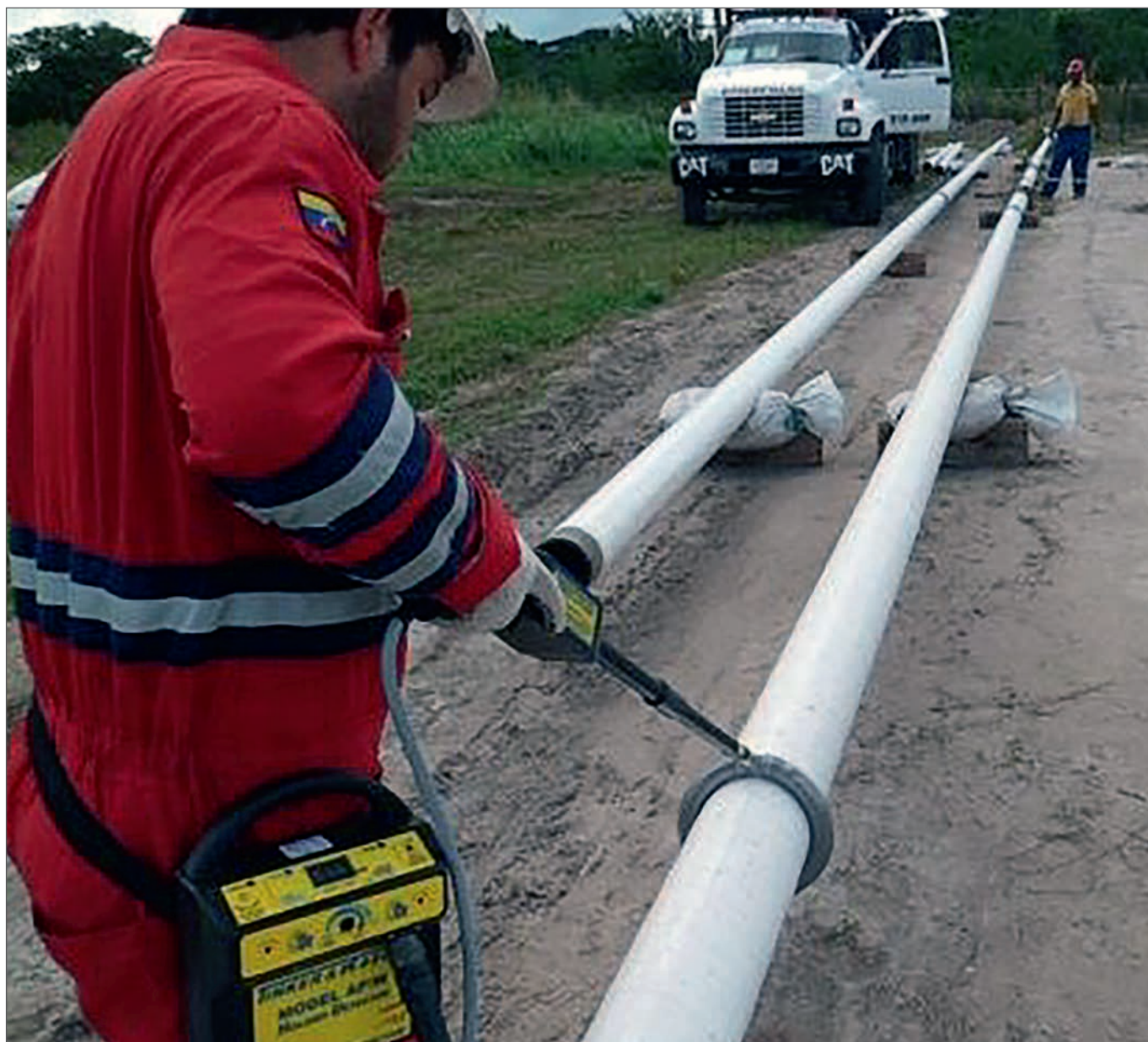
Inspector tests for holidays on a section of pipe using a full spring electrode. Source: Tinker and Rasor
