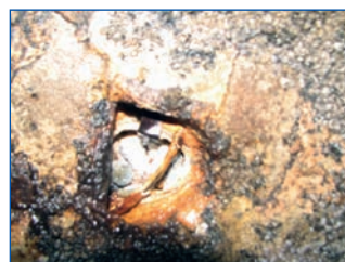
Figure 11. Example of acidification induced deterioration to pile anode cable insulation (typical).
