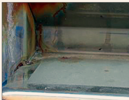
Figure 2: Corrosion on inner weld of stainless steel step.
