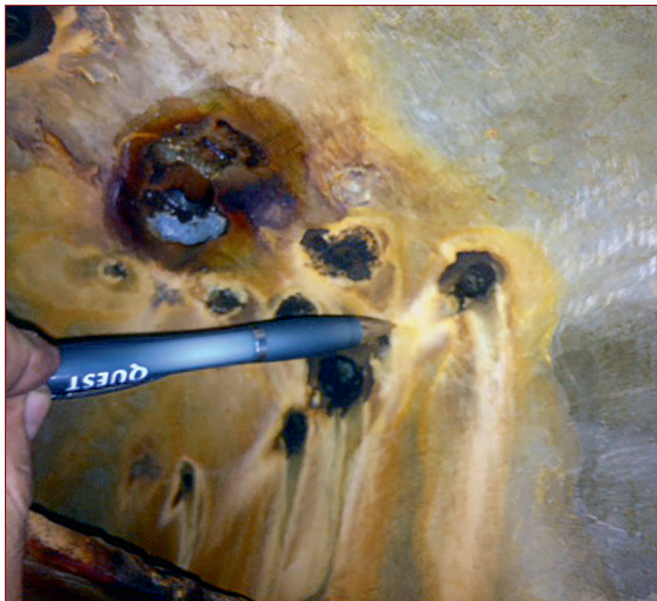
Figure 4. Deep pits in the case of a grade 5A superduplex low pressure pump.
