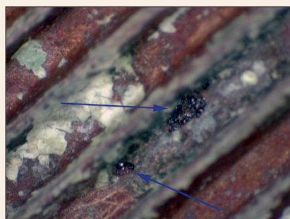
Figure 4. Pits that were beneath the adhered deposits on the Cu tube, 32 \times original magnification. Reproduced with permission from NACE International, Houston, TX [102].
