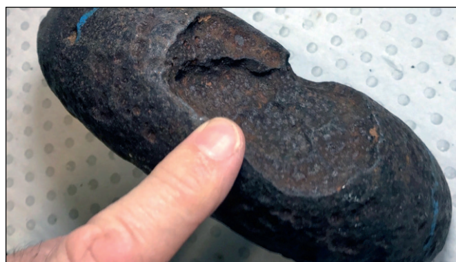
Part of a 76 mm diameter steel mooring chain link showing some of the severe corrosion found as part of the SCORCH project.
