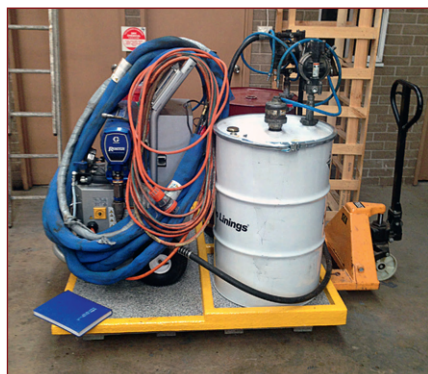
A Rhino Linings high-pressure, plural-component spray machine on a travel pallet.
