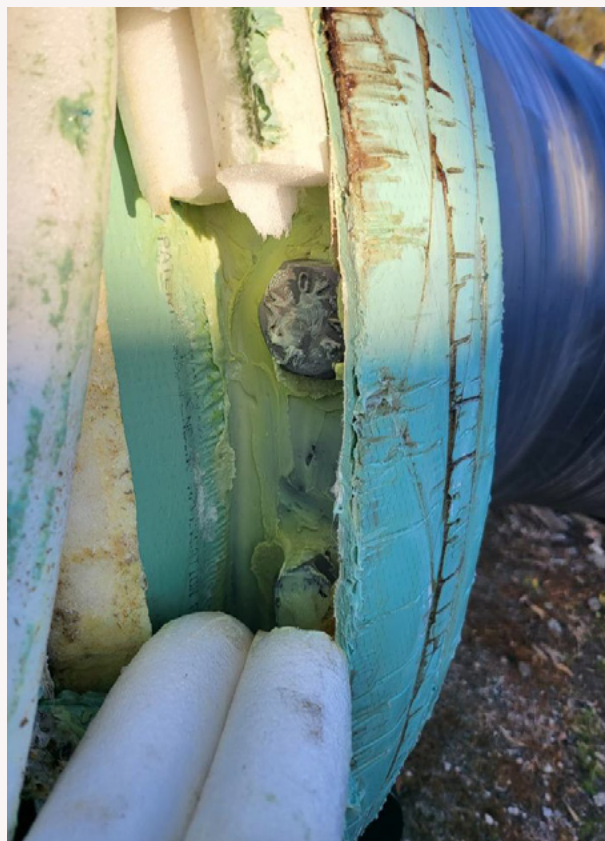
Figure 7: Previous foam roll insert backing system used in combination with PIB paste, no corrosion of steel
