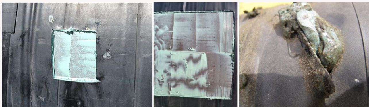
Figure 6: Inspection windows during condition assessment of steel pipe and self-healing example.
