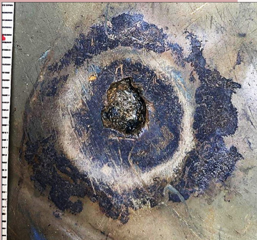
Figure 3: Evidence of AC corrosion on pipeline with visible arcing burn marks, metal loss of approx. 5mm, found on site.
