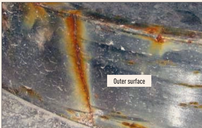
Figure 3: Crack initiation on the outside surface of the impeller wear ring.
