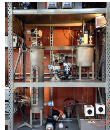
Feed blending and Monoethylene Glycol (MEG) pretreatment section of the MEG regeneration and reclamation facility.
