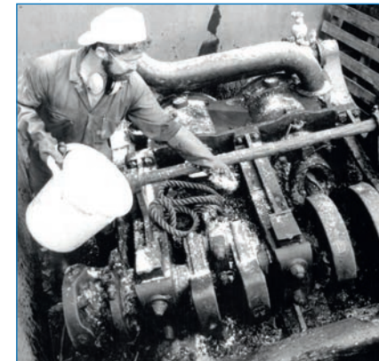
Spreading NaOH pellets on the Xantho engine in 1990.
