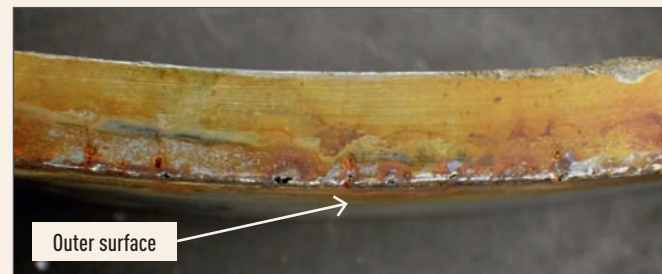
Figure 6: Corrosion pit on end of the wear ring which faced the impeller.
