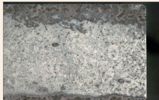
Figure 8: Cross-section through a non-failed ring showing the carbon rich zone at the outer and inner surfaces of the ring. The outer surface is orientated at the top of the picture.
