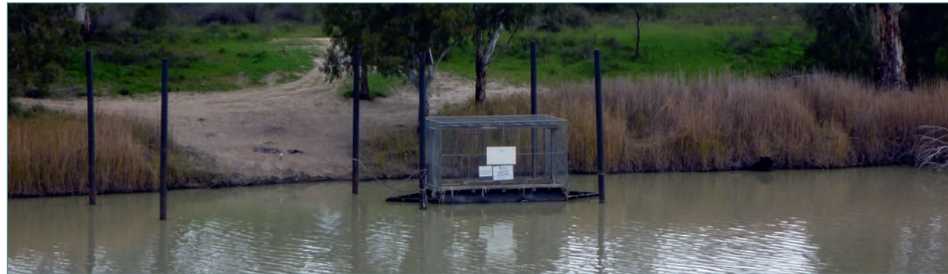
River Murray Pontoon used for river exposure samples.
