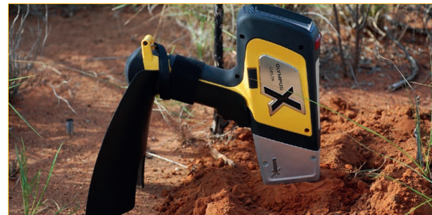
The compact, lightweight Delta Element hand-held XRF analyser from Olympus.
