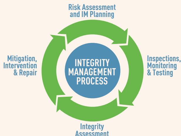
Figure 3. Pipeline Integrity Management Process (DNV RP F116 [4]).
